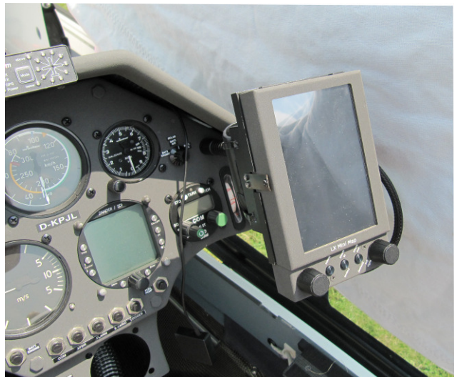
Out of panel installation after using of existent PDA support
