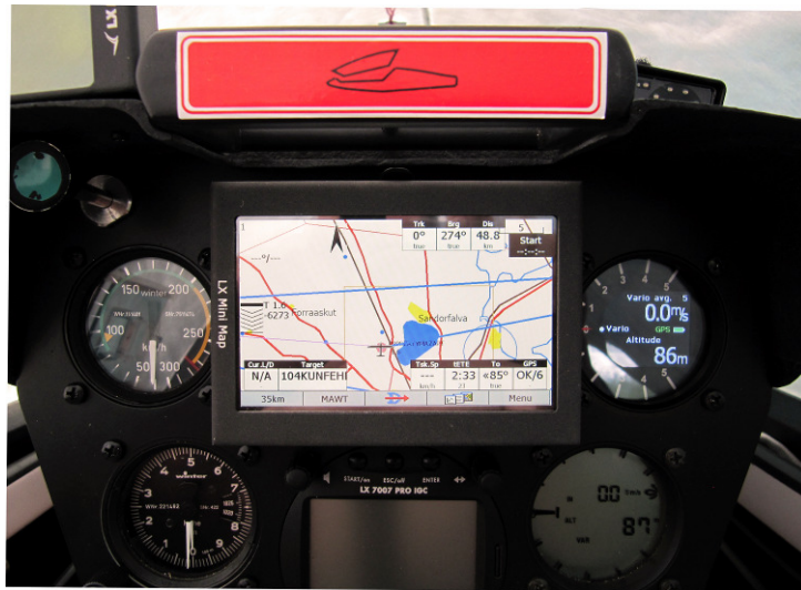
On panel installation controlled by LX Remote stick
