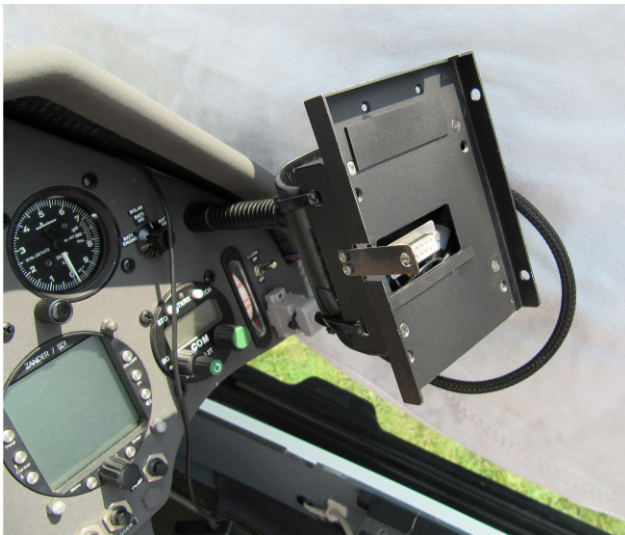
Out of panel installation after using of existent PDA support
