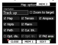
If **Zoom to target** is checked the zoom will be automatically adjusted so that the target point is always visible. Maximum zoom is 200 km and minimum zoom is 1 km. The check boxes will turn on or off the following items:
