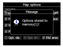
Press button **MEM 1** for a long time. A message "Options stored to memory (1)" will be displayed and the settings are stored. Change the settings a little bit. Press button **MEM 2** for long time. A message "Options stored to memory (2)" will be displayed and the settings are stored to memory location 2. Now short pressing of **MEM 1** will invoke the saved settings from memory 1.
