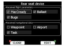
Data is divided into two groups; flight parameters and navigational data. If a specific value is checked this value will be automatically be received from the other device.
