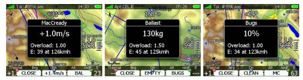
Use the lower-right knob to modify the MacCready setting. In the middle button there is a suggestion for the MacCready setting which is based on the last four thermals. Additionally to the selected MacCready value an overload factor is also shown together with the calculated glide ratio with corresponding speed.
