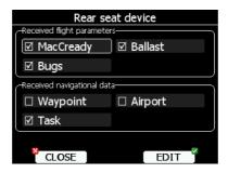
Data are divided into two groups; flight parameters and navigational data. If a specific value is checked this value will be automatically received from the other device.
