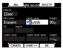
Press the **CHAR>>** button to advance the cursor to the next position. The cursor can also be moved to next position using the bottom-left knob. Rotate it clockwise to move forward. **The Abc** button is a toggle button and will change the letter case. Press it to toggle modes.
