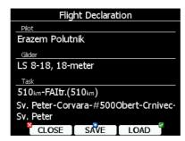
On the screen pilot, glider and task information are shown. Press the **SAVE** button to save the declaration onto a SD card or USB stick. Press the **LOAD** button for loading.
