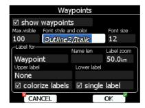
Turn the lower-right knob (page-selector) to change the font style. Text is also rendered in the selected font style. Turn the lower-left knob (zoom-selector) to change the font colour.
