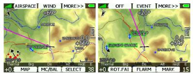
Press the **MORE>>** button to see more options. If the remote stick is available the behaviour is slightly different. When the check button is pressed on the remote stick a menu will appear instead of the button functions.
