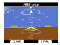
Place you glider in levelled position and press LEVEL button. You can also modify pitch only, if you rotate PAGE UP/DOWN rotary knob.
