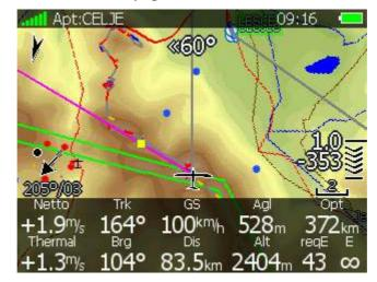
The additional items are the current net vertical speed, current track, ground speed, height above ground and optimised distance.
