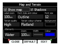
Check the **Show map** item to enable map displays in the navigational pages. If this item is unchecked no map will be displayed. Check **Shadows,** if you terrain to be shaded. The **Label zoom** value defines up to which scale of zoom city names are visible. 100km means the whole width of the screen represents 100 km. The user can also modify size, font style
