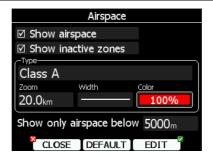
Rotating the zoom selector changes colour transparency. Transparency is very important for fill colours which are used for airspace zones, observation zones and FAI area. If a fill colour is not transparent (0%), all other map items will not be seen through it. If a fill colour is 100% only the solid border will be drawn.
