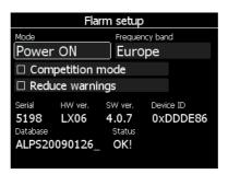
**Device ID** shows the Flarm unique ID, which is transmitted to other FLARMs. The Flarm status message is normally OK. In case of any errors or warning an error message will appear. The user can change the operation mode of Flarm unit, frequency and enable/disable competition mode.
