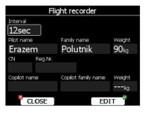
Select the recording interval and enter the pilot name. Pilot weight is important if ballast is specified in kilograms of water (see Chapter 5.1.11). If the LX8000 is used in two-seat aircraft the name of the copilot may also be entered.
