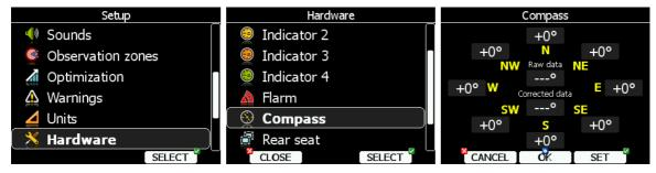
1. Orient the glider to face north. The **N** label will be automatically highlighted.
