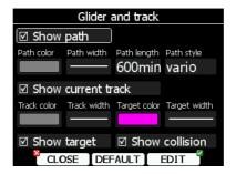
Check the **Show path** item if you want to see the flown path. **Path length** defines how much of the flown path will be shown. The maximum recommended length is 60 minutes. The path can be coloured using:
