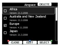
Select the required airspace and press **SELECT**. If a check mark is shown in front of an airspace item, this airspace file will be shown in the graphics and used for proximity calculation, when enabled.
